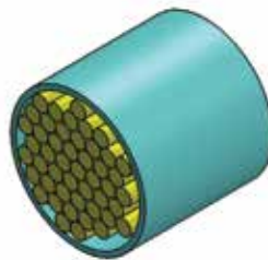
Duct containing 48 x Ø 3mm cable
