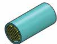
Duct containing 48 x Ø 1.2mm cable
